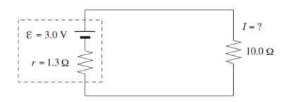
8. What is the terminal voltage of the battery in the circuit shown?
