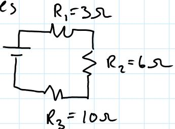
$$\begin{aligned} R_{\text{eq}} &= R_1 + R_2 + R_3 \\ &= 3\Omega + 6\Omega + 10\Omega \\ R_{\text{eq}} &= 19\Omega \end{aligned}$$
