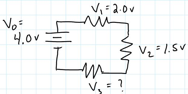
$$V_0 = V_1 + V_2 + V_3$$
