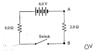
The switch in the above diagram is open. What is the potential difference  $V_{AB}$  across the  $2.0 \Omega$  resistor?
