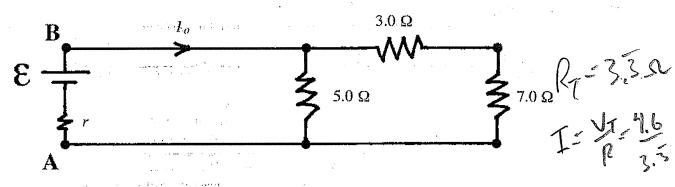
The EMF of the battery above is 6.00 V, and the terminal voltage  $V_{AB}$  is 4.60 V.
