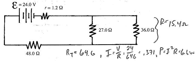
10. If the EMF of the battery above is 24.0 V and its internal resistance r is 1.2  $\Omega$ , what power is dissipated in the 48.0  $\Omega$  resistor? 6.6 W
