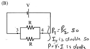
The power dissipated in circuit (A) in resistor R between 1 and 2 is P. In circuit (B) the same source voltage is used, but an identical resistor R is added in parallel with the first resistor. How much power will be dissipated between 3 and 4?
