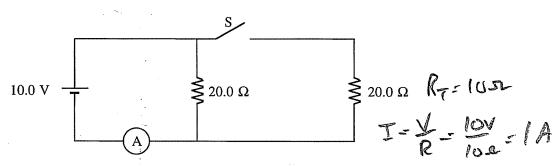
1. The current through A is 0.50 A when the switch S is open. What will the current through A be when the switch S is closed?
