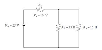
4. In the following circuit, what is the power loss in the battery?
