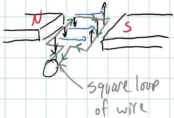
The magnetic force causes the loop to twist. If the loop is allowed to spin & the current is reversed  $\frac{1}{2}$  way thru, the loop could spin continuously (an electric motor)
