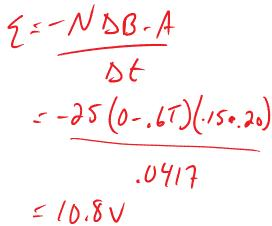
If the coil rotates  $90^{\circ}$  in  $4.17 \times 10^{-2}$  s so that its plane is now parallel to the magnetic field, what average emf is induced during this time?
