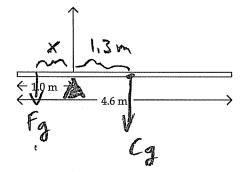
7. The motorcycle shown has a mass of 200 kg and a wheel base of 1.8 m. If the rear wheel exerts a 1 200 N force on the ground, find how far the motorcycle's centre of gravity is located from the front wheel.
