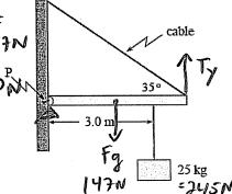
b) What is the magnitude of the horizontal component of the reaction force of the wall on the beam at the hinge P?
