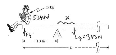
$\Sigma T = O CWT = CCWT$   $(539N)(1.3m) = (343N) \times \times = 2.0$  $2:Om+1.3m = 3.3m ( \frac{1}{2} \text{ the length,})$
