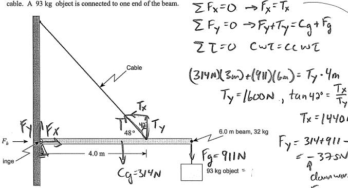
Fy= 314+911-1600 =-375N What is the magnitude of the horizontal force  $F_h$  that the hinge exerts on the beam? (7 marks)
