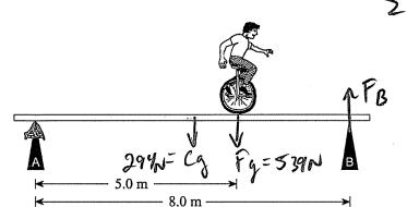
$\Sigma F_{y}=0 \Rightarrow F_{x}+F_{y}=C_{y}+F_{y}$   $\Sigma T=0 \quad (wT-Ccwz)$   $B \quad (294N)(4)+(539N)(5)=F_{y}(\delta a)$   $F_{y}=484N$   $F_{x}=294+539-484N$
