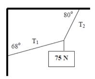
13. A 75 kg traffic light is held stationary midway between two supports, as shown in the diagram below. What is the tension in the cord?
