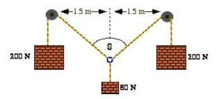
12. Find the tensions  $T_1$  and  $T_2$  in the ropes shown in the diagram.
