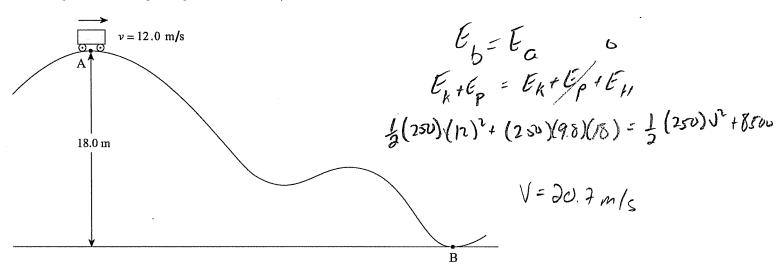
What is the speed of the roller coaster at point B at the bottom of the hill if 8 500 J of energy is transformed to heat during the journey? (7 marks)
