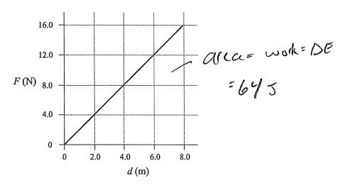
If the object was initially at rest, what is its kinetic energy after travelling 8.0 m?
