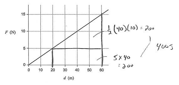
What is the work done in moving the object from 20 m to 60 m?
